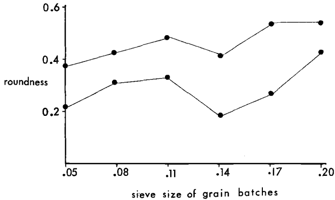
FIG. 5—Graphical representation of Powers roundness values versus size of sand grains.
